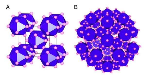
Periodic and quasiperiodic arrangement of atoms. A) An example of cubic unit cell in which the icosahedron occupies the corner and body-centered positions.Pink balls indicate atoms. B) An example of the Tsai-type icosahedral quasicrystal. The fivefold rotational symmetry and the self-similarity may be observed.
