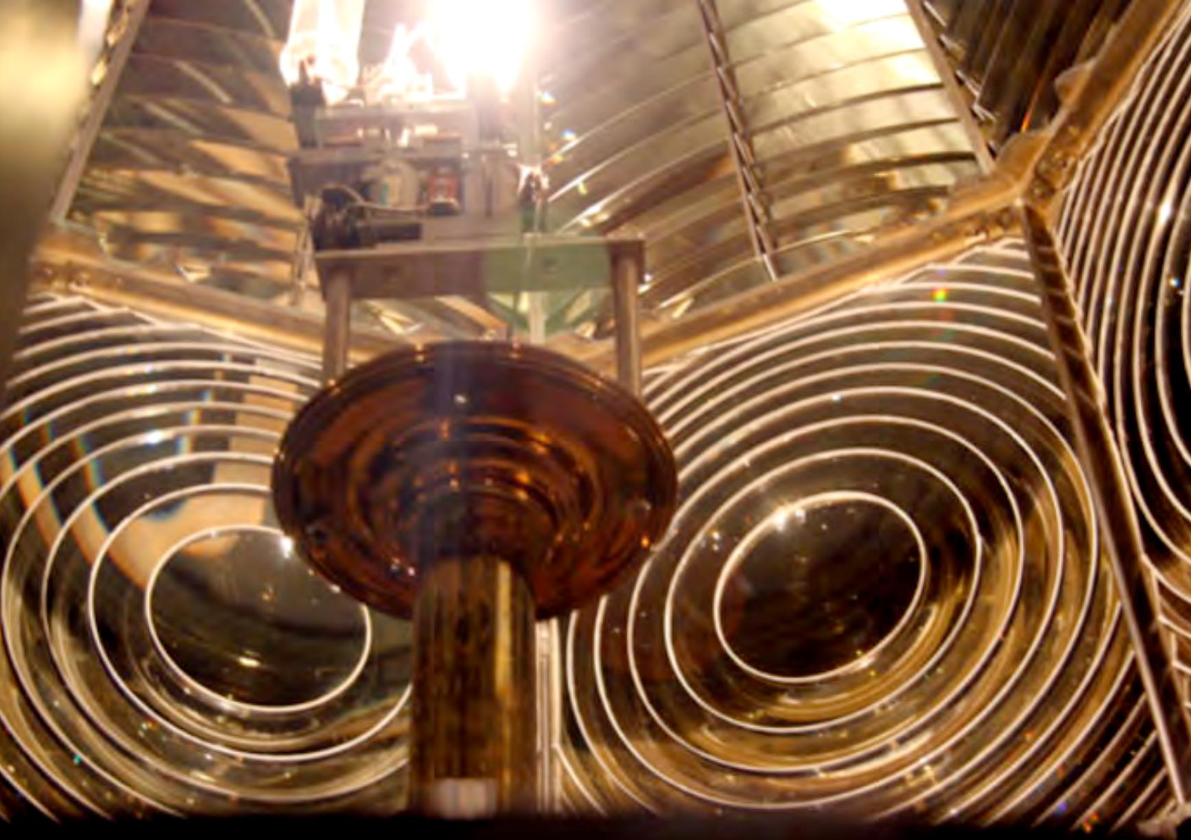
Fresnel lenses focus beams of high-intensity light
